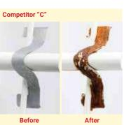
See www.erico.com for the terms of the Armour 10-year limited warranty. \* Salt-spray testing test method: ASTM B117 / DIN 50021; Cyclic corrosion test method: GM 9540P.
